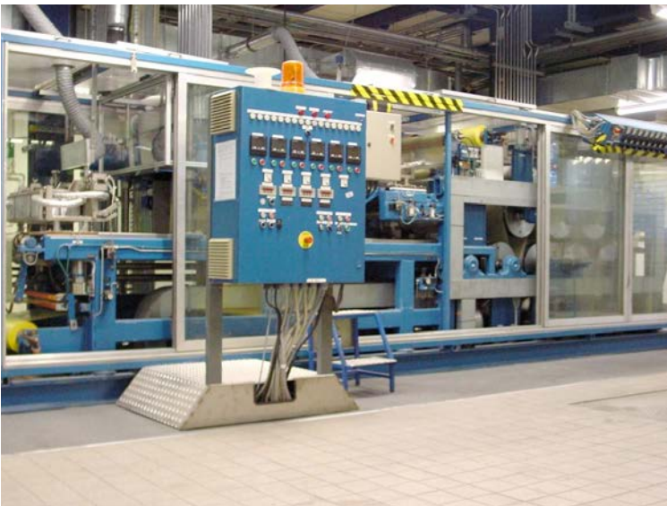
■ Fully monitored SMC line used for product development and process quality improvement.
