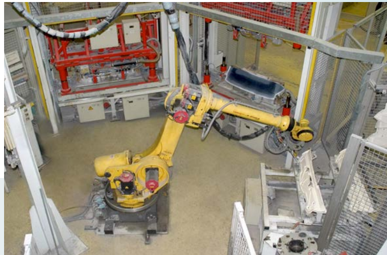
■ Pick and place robot transfers spoiler mouldings
