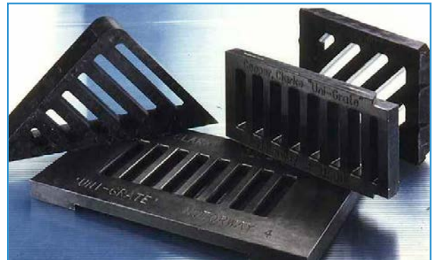
SMC grids. As well as being lighter than cast iron equivalents, SMC grids, gratings and manhole covers also have no scrap value so there is no danger of theft. The same applies to motorway road signs where SMC is being used to replace aluminium for the same reason.
